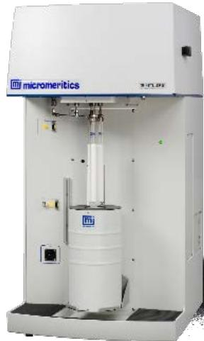
BET surface measured with Micromeritics 3Flex surface analizer
