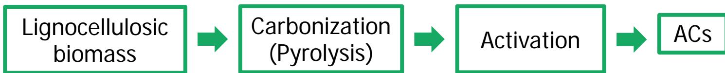
**Carbonization:** Pyrolysis at 400-600°C for 1-2 hours
